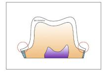
The ceramic shoulder margin of the zirconium oxide framework has the function of supporting the silicate ceramic veneer structure. The framework structure here takes on the function of a prepared tooth stump (= a shoulder with a circumferential chamfer or a rounded inner angle). Consequently, the tested and tried principles can be used for the design of silicate ceramic CAD/CAM restorations.
